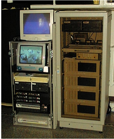
Figure 7: The technics rack: To the left the show-control system can be seen, in the upper right there are two DVD players, at the bottom the 4 PCs running the game engine
