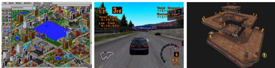
Figure 2: (a) isometric projection, (b) central perspective with one, (c) perspective with three vanishing points
